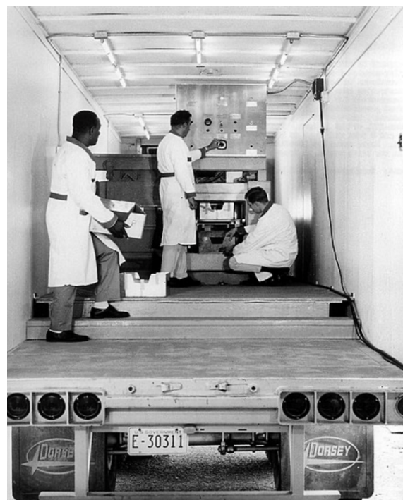
A Portable, Food Irradiation Machine. 1968 photo from Wikipedia
